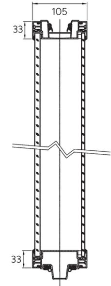
Horizontal Section Through Standard Panel
